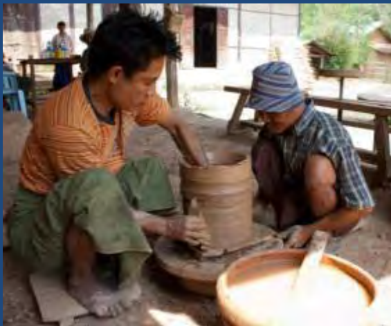
Pottery process of making an A1 improved cook stove (ICS)
