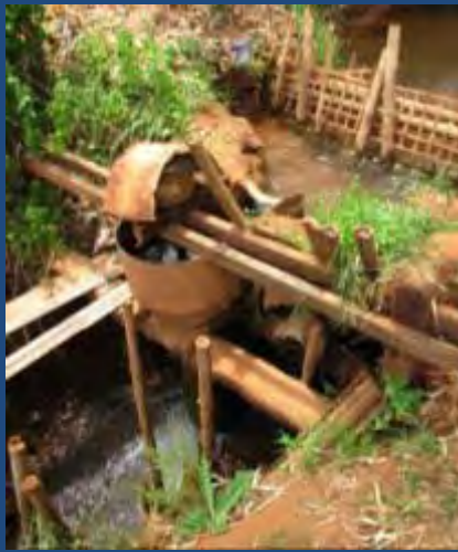
Surprisingly functioning: low-cost pico hydro system integrated in a drop-structure of the irrigation
