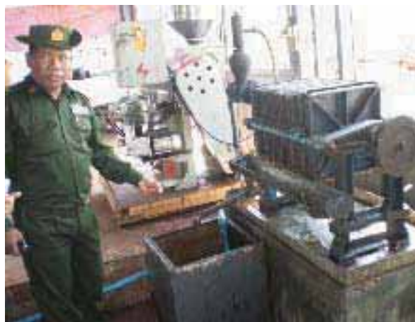
Figure 23: Jatropha Crude Oil Expeller in North-Eastern Military Command, Lashio
