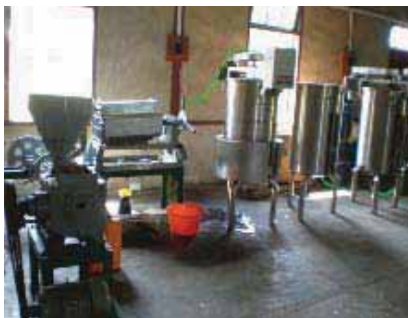
Figure 22: Pilot Batch Type Jatropha Crude Oil Expeller and Processing Plant, Hline Tet Farm
