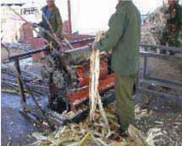
Figure 28: Rollers at the Demonstration Ethanol Plant
