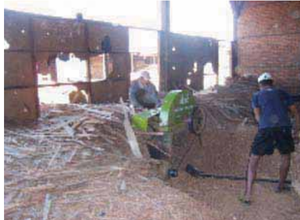
Figure 35: Making Wood Chips from Plywood Waste at JLC, Mandalay
