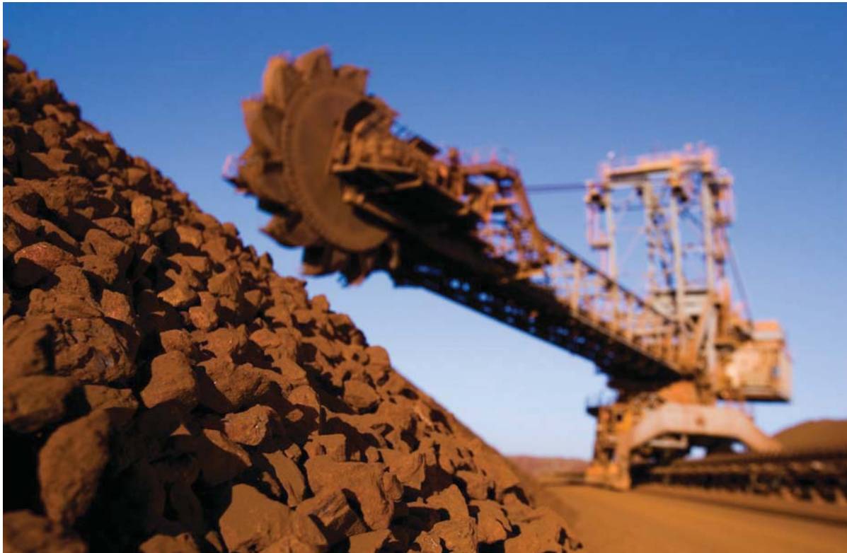
A stack reclaimer with a pile of iron ore at the Rio Tinto Parker Point ship loading terminal in western Australia.
