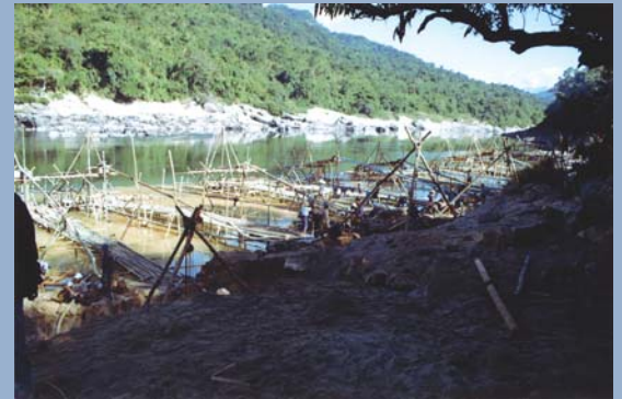
Photo 31: Gold mine pools and bamboo sluices on the eastern side of the river at Nawng Hkying (between the Confluence and Myitkyina).
