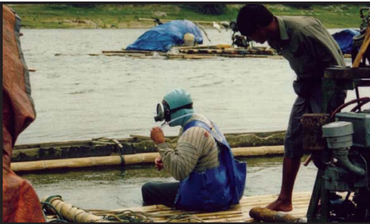
Photo 18: Divers on the Mali Hka spend up to eight hours per day under water working only with simple diving equipment.
