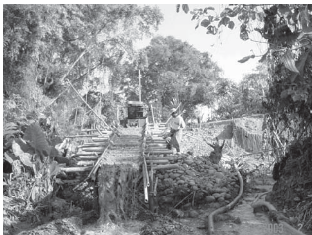
Photo 10: Sand and rock pumped or scooped from the river bottom passed through a sluice tray (in this case a simple bamboo sluice) with water in order to separate the gold containing sediments.
