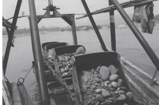
Photo 11: Bucket dredges operate in the river using belt driven buckets to scoop material from the river bottom.
