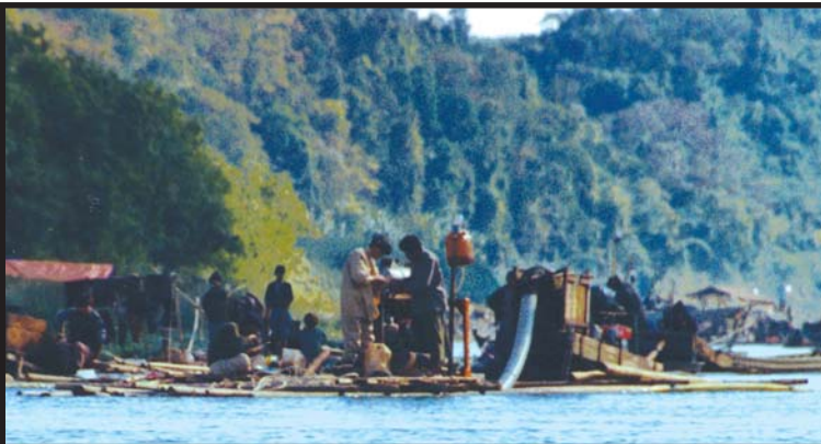
Photo 19: Suction dredges on the Mali Hka river use suction pumps driven by Jinma engines to suck up sand and gravel from the bottom of the river.
