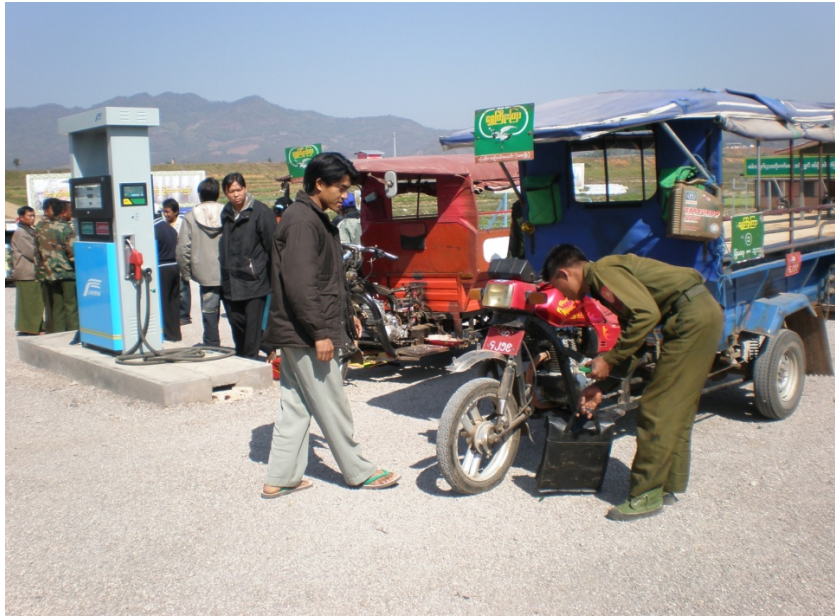
Military Engineer adjusting the fuel system of the motorbike for ethanol
