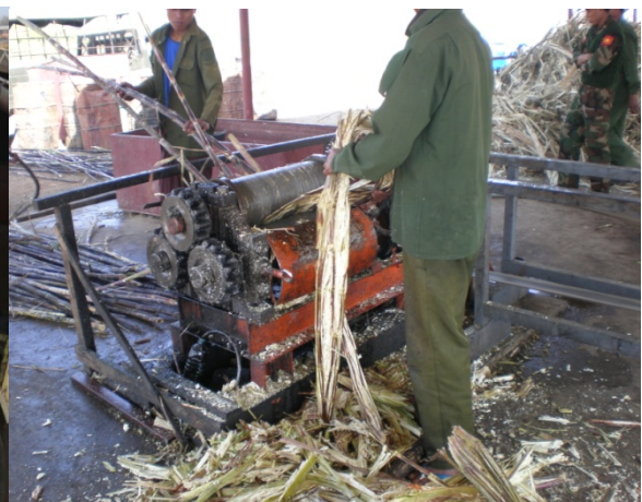
Rollers of the demonstration ethanol plant
