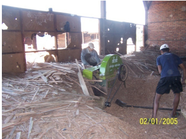
Making wood chips from ply-wood waste in JLC Company.
