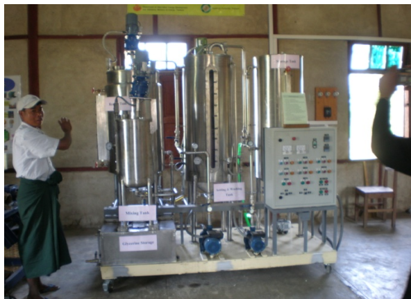
Pilot Jatropha Crude-Oil Expeller and Processing Plant (Continuous Type), Hline Tet Farm, MAS, Mandalay Division (23-2-08)
