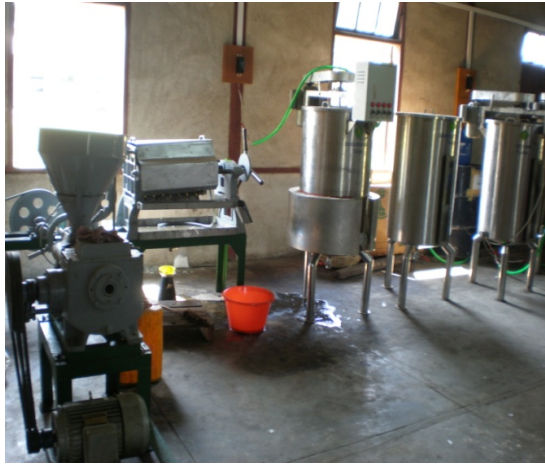
Pilot Jatropha Crude-Oil Expeller and Processing Plant (Batch Type), Hline Tet Farm, MAS, Mandalay Division (23-2-08)
