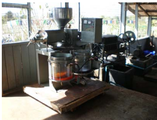
Mini Jatropha Refine Oil Processing Machine made in China, North-Eastern Military Command, Lashio, Shan State (25-2-08)
