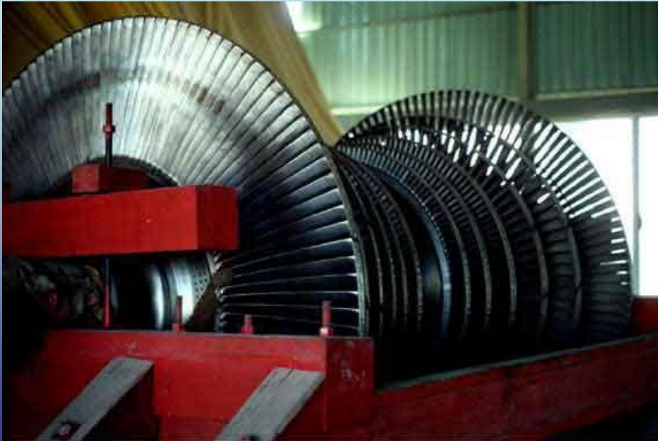
Turbine blades inside a geothermal turbine generator.
