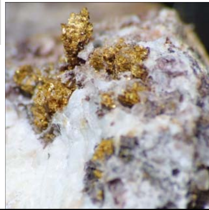
Segment of Au-bearing quartz vein on 950m level at Htongyi Taung, 40cm@11 g/t, looking SE.
