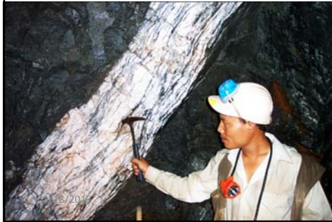
Segment of Au-bearing quartz vein on 950m level at Htongyi Taung, 40cm@11 g/t, looking SE.
